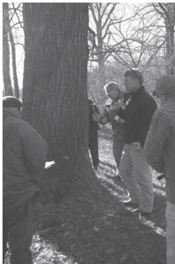
Dr. Luley shows a class how to test for decay using a mallet.
